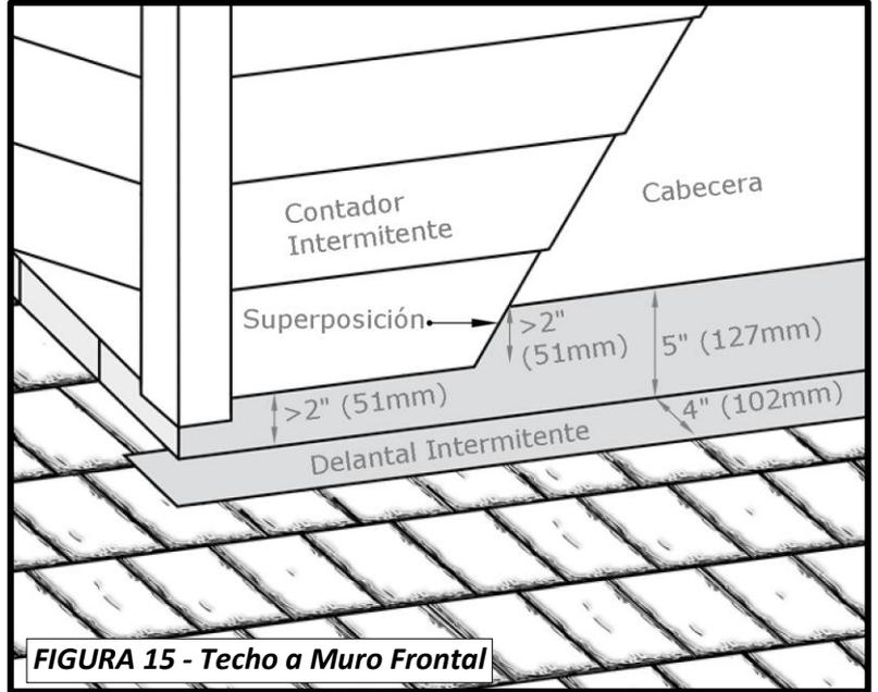
**FIGURA 15 - Techo a Muro Frontal**
